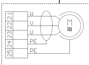
It is FUNDAMENTAL to connect the electric EARTH to the control board and the motor in order to obtain the correct operation of the control board and photocells !
